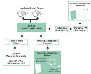
\*Up to 6 Remote Input Plates can be cascaded together for additional music/AV inputs.
